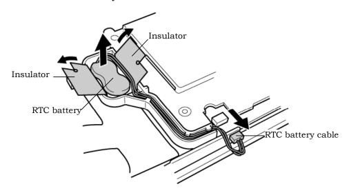
Figure 4-22 Removing the RTC battery
